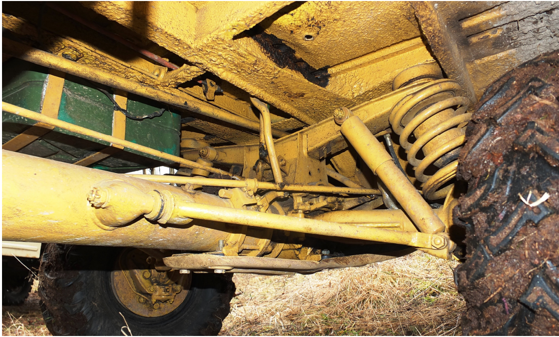
(here's a photo, by Linton, of the underside of John's Haflinger) Central tube chassis, coil springs, clever, but also simple and basic. Cool.
